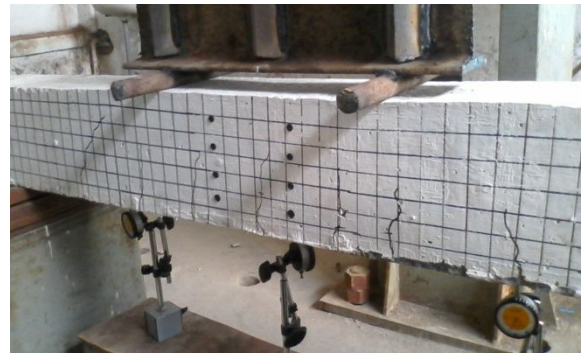
b) Crack pattern for Mix M4
